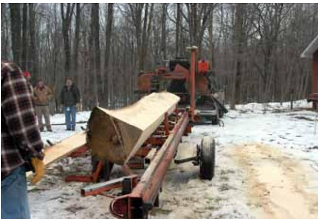
Ash logs can be milled on site using a portable sawmill.
